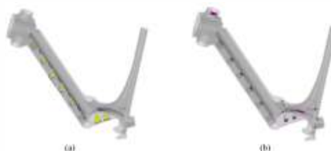
FIGURE 8 Solidification analysis of the frame: a) Last sections to solidify; b) shrinkage porosity prediction.
