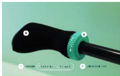
FIGURE 1 The developed grip and its features: (A) encoder and (B) vibrational motor.
