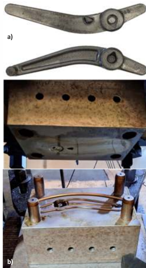
FIGURE 1 a) Safety system component of two-wheeler vehicles after forging; b) Tools (top and bottom dies) used in the forging process.
