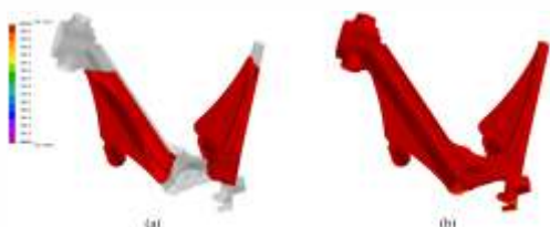
FIGURE 7 Filling analysis of the frame; a) beginning of filling b) end of filling,
