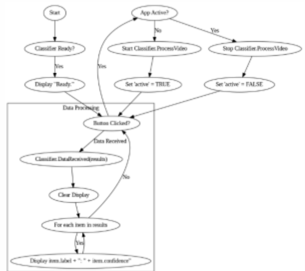
FIGURE 2 Flowchart 1: Operation Flow of the Driving Assistance App for Electric Scooters.
