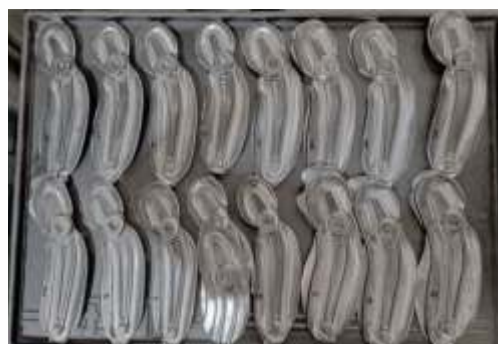
FIGURE 3 Examples of parts obtained after the forging process: A356 (top); 357 (bottom).
