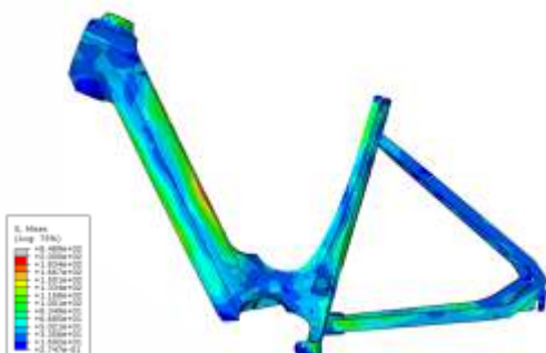
FIGURE 3 Falling frame - Impact test results according to ISO 4210.
